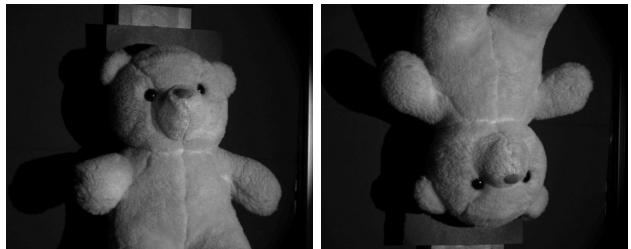
Figure 6: A reciprocal pair of images of the teddy bear; the second image is obtained by interchanging the position of the light source and camera.
