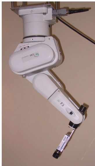
Figure 3.8: Camera mounted on the robot arm used to generate the translation motion.
