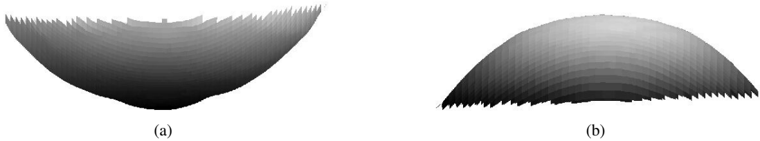
Figure 7.9: Reconstruction of the inner part (a) and outer part (b) of a spherical cap. (a) corresponds to the ping-pong ball section considered in this section, while (b) corresponds to the snooker ball considered in the previous chapter (see Fig. 6.7). Both models were obtained from integration of the normal field. Similar view points are considered for both objects. It is clearly visible that (a), which is concave, is not as well reconstructed as (b), which is convex. The errors in the first case are due to inter-reflections which corrupt pixel based intensity measurements.
