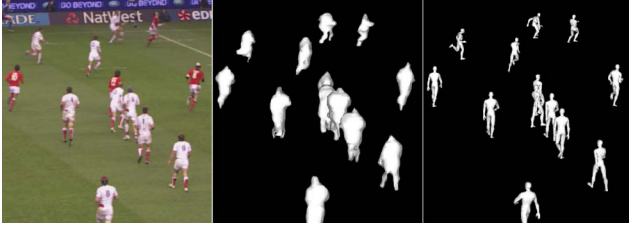
Figure 9. Left to right, the original input image, the resultant CVH and the final matched pose. Some synthetic players are mirror images of the original player, as left/right symmetry introduces an ambiguity that is difficult to resolve completely.
