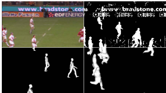
Figure 1. A split image depicting four stages of processing. Clockwise from the top-left - the original image, a segmented “key” separating the players from the background, a 3D reconstruction of the players and the final synthetic proxies of the players.
