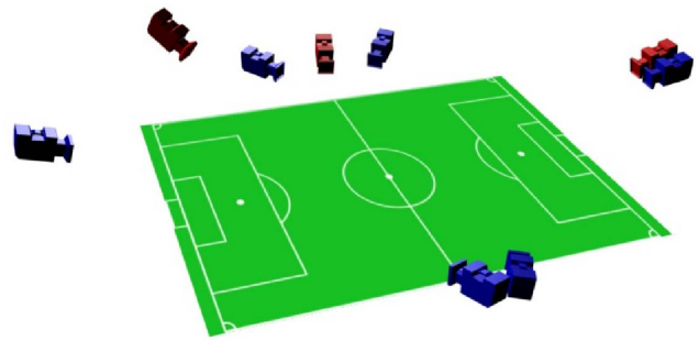
Figure 8. Arrangement of cameras used for the rugby data set. Static cameras are coloured blue while moving cameras are coloured red. Note that the static cameras are aimed at either one end of the pitch or the other, so that at any one time only 3 static cameras and up to 3 moving cameras are usable for reconstruction.
