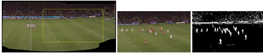
Fig. 7 Difference keying. The camera image (middle) is compared against a spherical panorama of the scene (left) giving the key (right).
