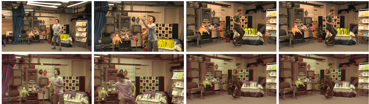
Figure 8. Sample images from the applications. Top: Scene augmentation. Bottom: Stereoscopic rendering, in red/cyan anaglyph format. Left: Juggler. Right: Unicycle2. Full video sequences are available at http://www.guillemaut.org/publications/11/Imre3DIMPVT11/videos
