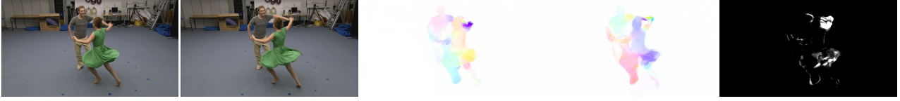
Figure 2. From left to right: a pair of consecutive input images, its forward and backward flow and a visualisation of the forward backward error map (for display purposes the error map has been normalised using histogram equalisation).
