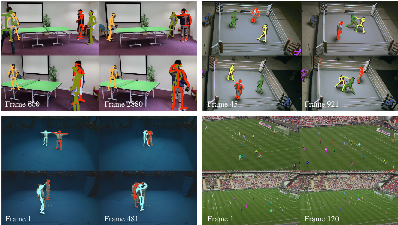
Figure 4: A selection of frames from the table-tennis, boxing, karate and soccer datasets showing results of 3D skeleton estimation plus tracking.
