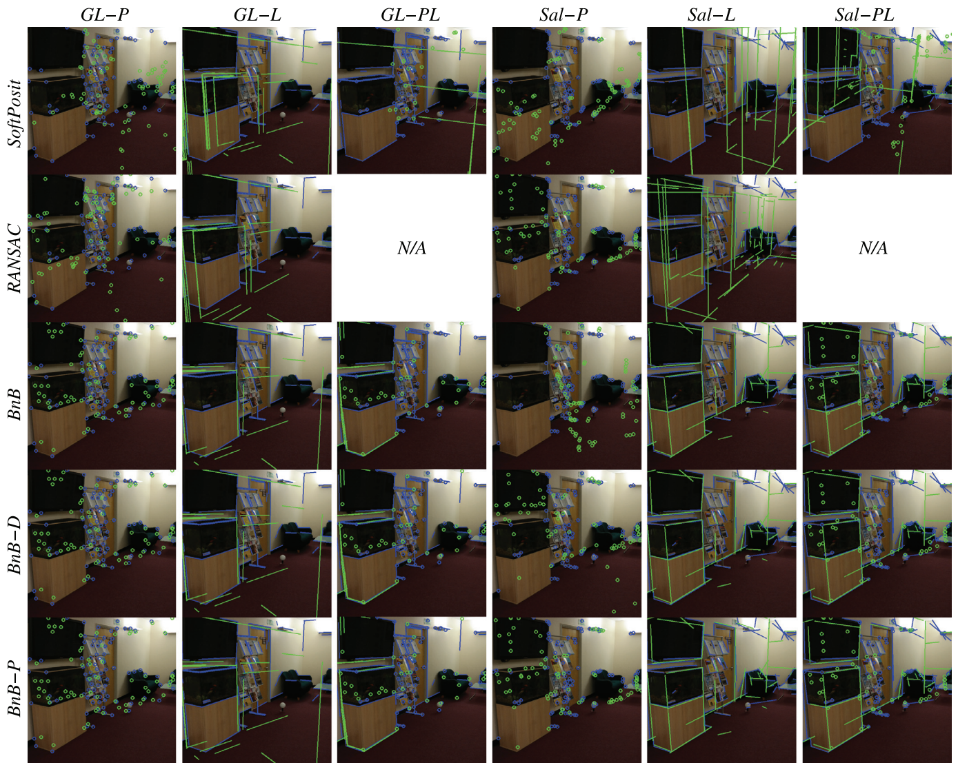
Fig. 9. Qualitative result for solutions returned using all methods on an image from Reception dataset. Blue features are 2D, green are 3D. (For interpretation of the references to colour in this figure legend, the reader is referred to the web version of this article).
