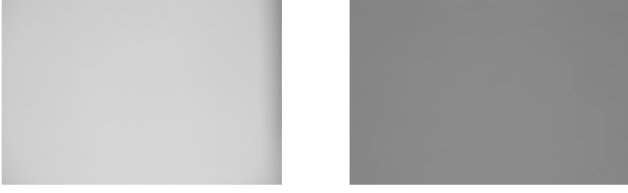
Figure 3. Calibration images of a uniform plane used for deriving average brightness focused at infinity (left) and at a focus setting (right). The observed change in brightness is purely a result of refocusing the camera. Images are white balanced and brightened for visualisation.
