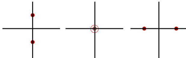
Fig. 2. Movement of the eigenvalues of  $\mathbf{J}^{-1}\mathbf{L}$  near a saddle-center transition, plotted in the complex  $\lambda$ -plane.
